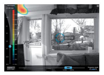
Having determined that the intake valve was the main noise contributor, this spot was covered up with a pillow to remove it from the overall noise field, and try to locate secondary sources. By filtering on a relatively high frequency band around 3 - 4 kHz, it was possible to filter out only the noise being emitted by small gaps and cracks. This produced two new possible weaknesses, one on the porch door, and another on the air valve above the window as seen in the image below.
