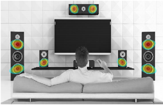
Fig. 3. Simulated image of eight point sources at frequency 3.5 kHz with ring array with all elements. Image shown with dynamic range 3 dB.
